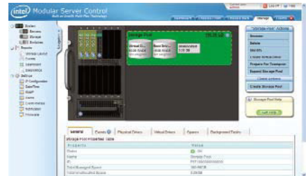
Under the Storage Configuration window, you can create storage pools and virtual drives, as well as map virtual drives to servers
