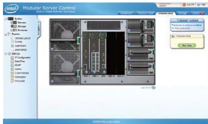
The back view of the chassis allows you to see the status of your modules and power supplies
